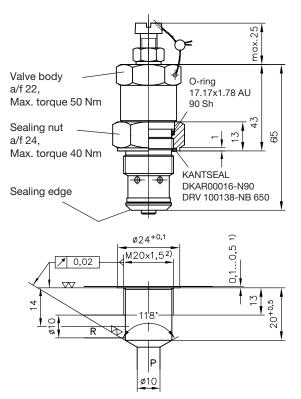
Mounting holes in the manifold may be blocked if required by tapped plugs, e.g. if uniform manufactured manifolds should be equipped with or without cartridge valve depending on application. For suited tapped plugs, see sect. 4.4 in D 7710 (pressure limiting valves type CMV 2)
