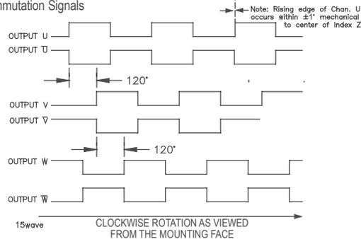
NOTE: ALL DEGREE REFERENCES ARE ELECTRICAL DEGREES. WAVEFORM SHOWN WITH OPTIONAL COMPLEMENTARY SIGNALS A, B, Z FOR HV AND OD OUTPUTS ONLY.
