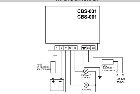
Devices must be provided for disconnection from the mains: for example, switches
