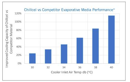
\*Tested in a NATA (National Association of Testing Authorities) accredited laboratory. Cooling capacity calculation based on AS2913, Breezair TBSI550 Cooler and inlet air temperature wb 22°C. Competitor evaporative media saturation efficiency assumed to be 80%.
