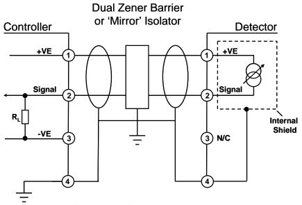
Diagram 4: Dual barrier schematic
