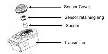
Diagram 7: Replacing plug in sensor
