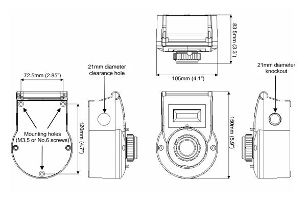
Diagram 2: Detector dimensions and mounting hole locations
