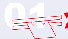
Actuating the footswitch closes the sealing bars and starts the vacuum-sealing process: The vacuum pump switches on and evacuates the air from around the product.
