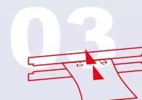
The sealing bars then fully close and seal the packaging material. After the sealing process, the sealing bars open automatically and the sealer is immediately ready for the next pass.<sup>1</sup>
